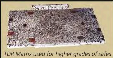
TDR Matrix used for higher grades of safes
